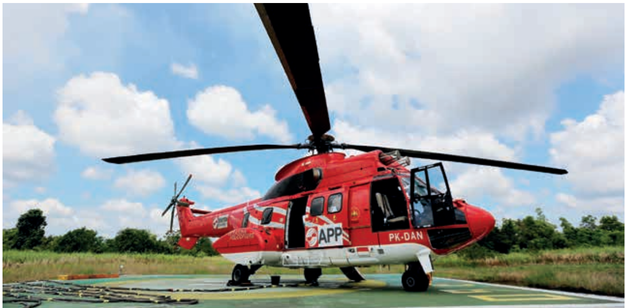
► Helikopter Super Puma untuk water bombing . Super Puma Helicopter for water bombing.
